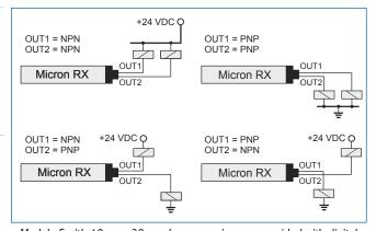
Models C with 10 mm, 30 mm beam spacing are provided with digital outputs 0-24VDC Push-Pull type.
