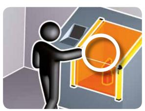
The resolution is maintained (up to 40 mm) in the junction between the 2 protected areas
