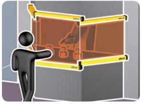
Example of series connection of one master and two slave light curtains for the protection of three sides of the machine
