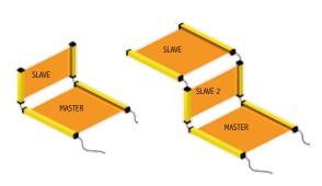
Master, Slave models permit series connection of up to three light curtains and combined detection of hand and presence of a person or of more sides of the machine
