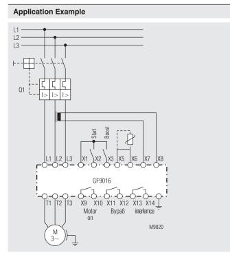
Softstart and softstop function from 25 kW withcontrolled current on start up.
