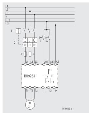
230/400 V AC-Mains AC/DC 24 V control voltage
