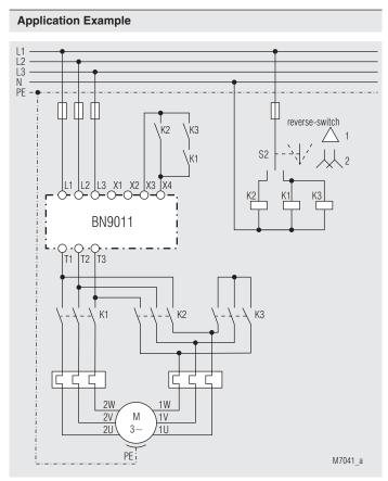
BN 9011 connected to a 3 phase multi-pole (Dahlander) motor with reversing
