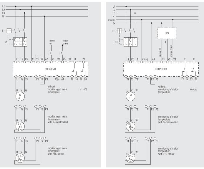
BI 9028/5\_ \_softstart and brake function switching via separate control inputs, auxiliary voltage  $\rm U_{H}=AC$  230 V
