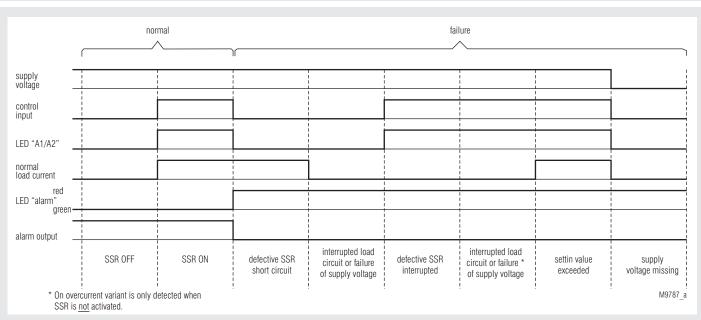
Normal operation and failure status
