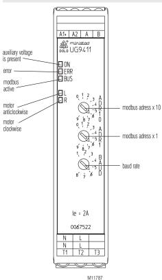
Position 7 Potentiometer 1 2 3 4 5 6 8 BAUD Baud rate 1200 2400 4800 9600 19200 38400 57600 115200 Baud Response < 50 < 25 < 12 < 10 < 5 < 5 < 5 < 5 Time ms ms ms ms ms ms ms ms
