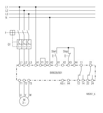
Fig. 2: Schematic diagram for softstart-brake combination
