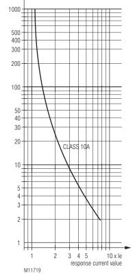
Trigger characteristics Motor overload protection
