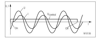
Current and voltage characteristics in the AC system with zero-voltage switching solid-state contactor
