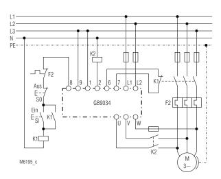
Fig. 1: Schematic diagram for a motor with electronic braking K1 = mains contactor; K2 = braking contactor
