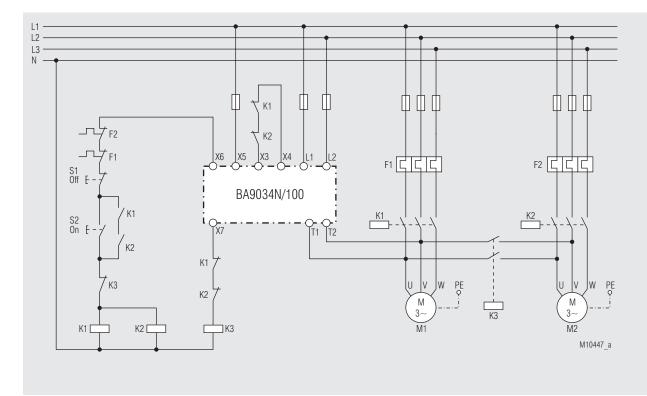
BA 9034N/100 simultaneous braking of 2 motors in parallel connection for lower motor loads
