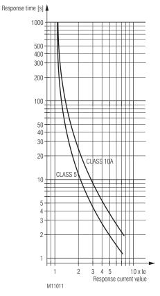
Trigger characteristics Motor overload protection
