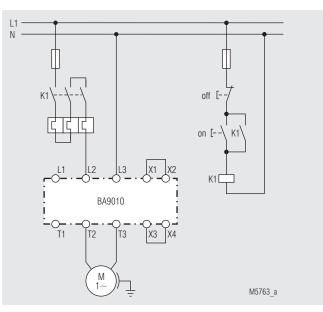
Softstart of a single phase motor on 230 V AC supply
