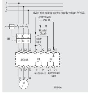
Softstart- and softstop function (Devices with external control voltage))
