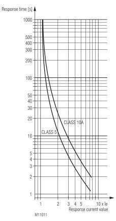
Variant / \_ \_ 1: Trigger characteristics Motor overload protection
