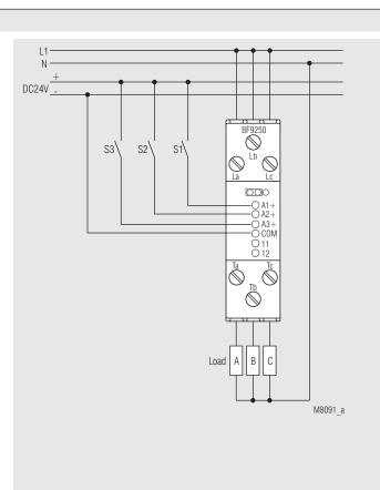
BF 9250.03/004 3 semiconductor contactors in one housing control 3 different loads
