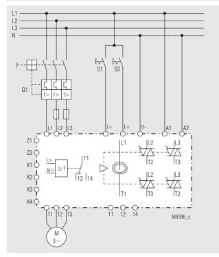
BH 9255 with A1/A2 = AC 230 V and control input AC/DC 80  $\dots$  230 V
