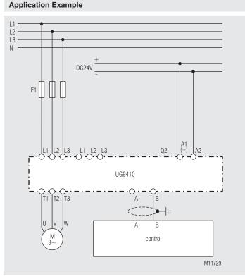
Motor control with UG 9410 and PLC via Modbus
